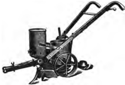
Improved cotton drill with fertilizer attachment
